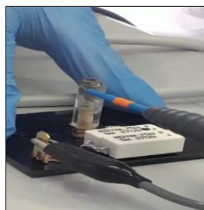
Figure 2 - Application of the electrical procedure on the surface of an E. faecalis contaminated implant in homemade polystyrene-based chambers.
