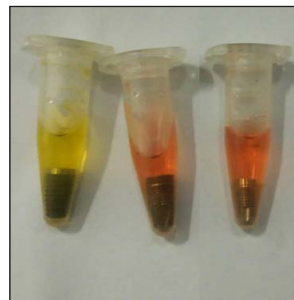
Figure 4 - Chromatic observation in the macro-method procedure after 72 h. First vial from the left: sample of BTA reagent from untreated implant; central vial: BTA reagent from the implant after electrical treatment; last vial on the right: negative control.
